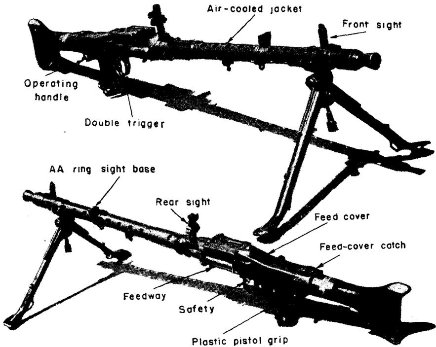
Figure 33.—Two views of M.G. 34 on bipod mount.
