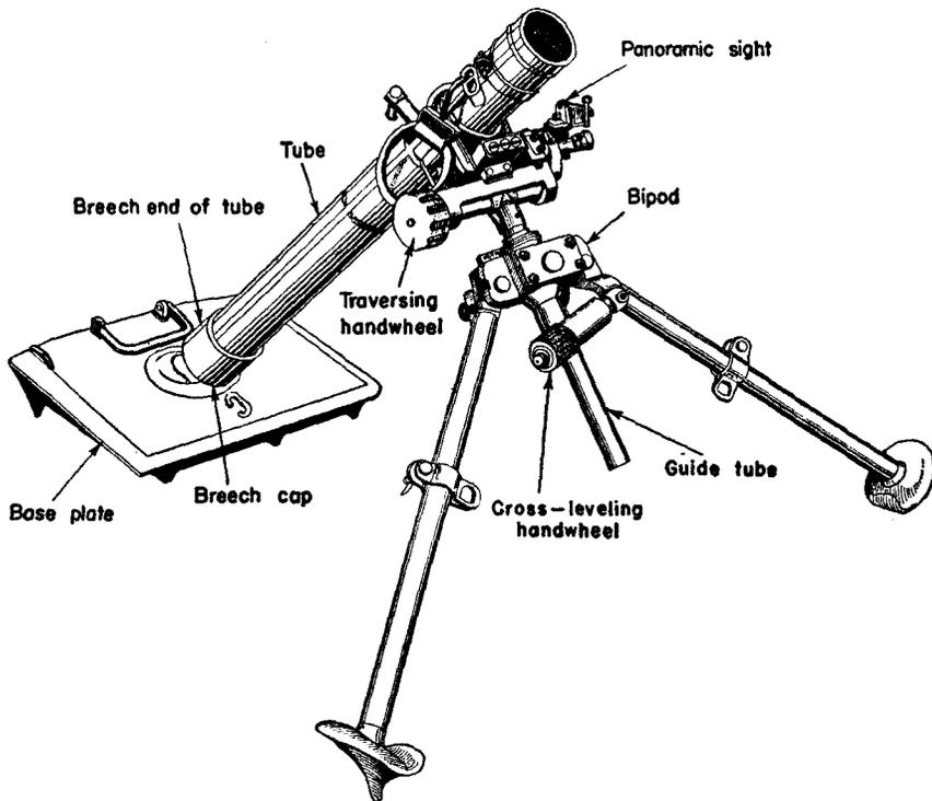
Figure 55.—Right view of 8-cm mortar, model 34.
