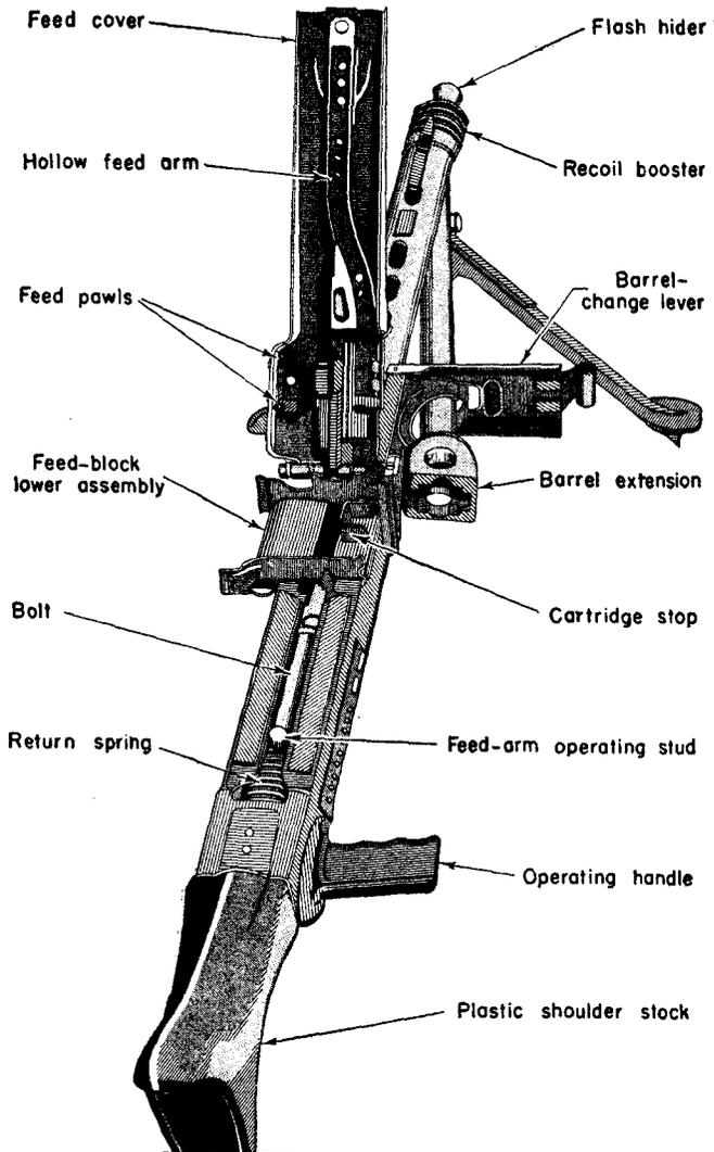
**Figure 51.—M.G. 42, showing method of operating barrel extension.**
