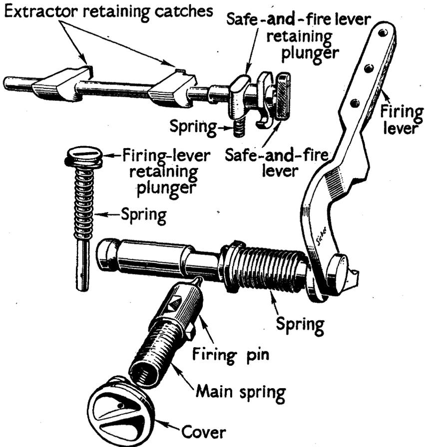
Figure 74.—Firing mechanism parts of 7.5-cm infantry howitzer.
