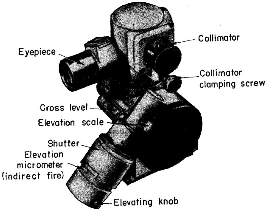
Figure 44.—Telescopic sight for M.G. 34 (rear view).
