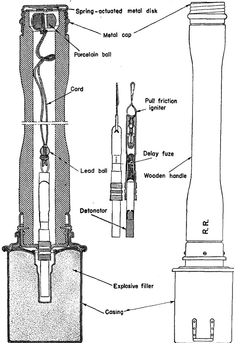
Figure 25.—Sketch of *Stielhandgranate* 24 (stick hand grenade, model 24), showing outside and cross section of grenade and fuze. (The cross section of the grenade is drawn to a larger scale than the scale of the sketch of the outside view.)
