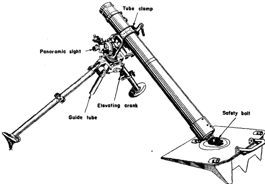
Figure 56.—Left view of 8-cm mortar, model 34.
