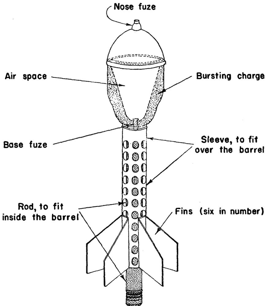
Figure 62.—Stick bomb for use with 3.7-cm Pak.
