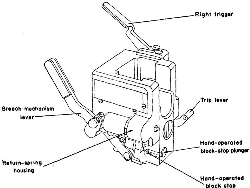
Figure 61.—Breech mechanism of 3.7-cm Pak
